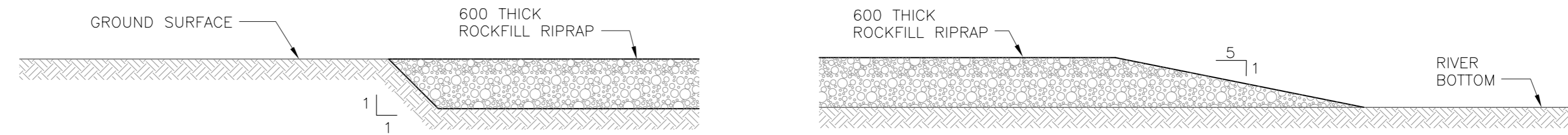
RIPRAP TRANSITION SUB CUT ABOVE UWRL RIPRAP TRANSITION BELOW WATER SCALE: NTS
